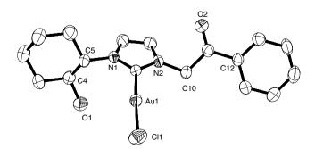
Fig. 3. ORTEP of 1c with thermal ellipsoids drawn at 50% probability level. Selected bond lengths (Å) and angles (°): Au–C(1) 1.991(4), Au–Cl(1) 2.2921(11), N(1)–C(1) 1.344(5), N(2)–C(1) 1.356(5), C(1)–Au–Cl(1) 177.53(10), N(2)–C(1)–N(1) 105.9(3).
